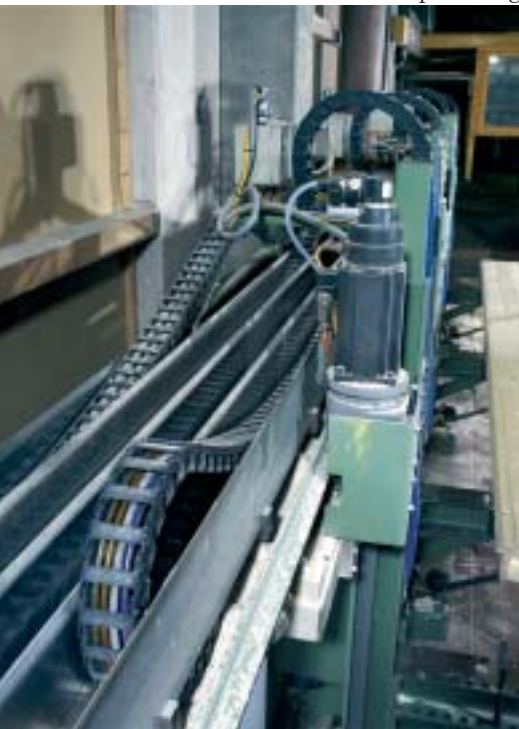
In the four X-axes of the Lignamatic, Kabelschlepp cable carriers of the Mono series, type 0450.41 with a length of up to 48 meters are used. The illustration shows the cable carrier in a gliding arrangement.
